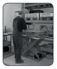
A lifting table eases manual handling and optimizes efficiency.
